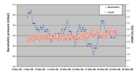
Variability of CH4 concentration in a mine ventilation shaft
