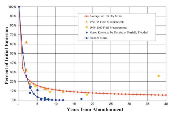
AMM emissions decline curves for dry vs flooded coal mines.
